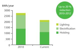
The calculation is based an elevator speed of 1.6 m/s, a load of 1000 kg, 200,000 starts/year, a travel height of 45 m and 15 floors
